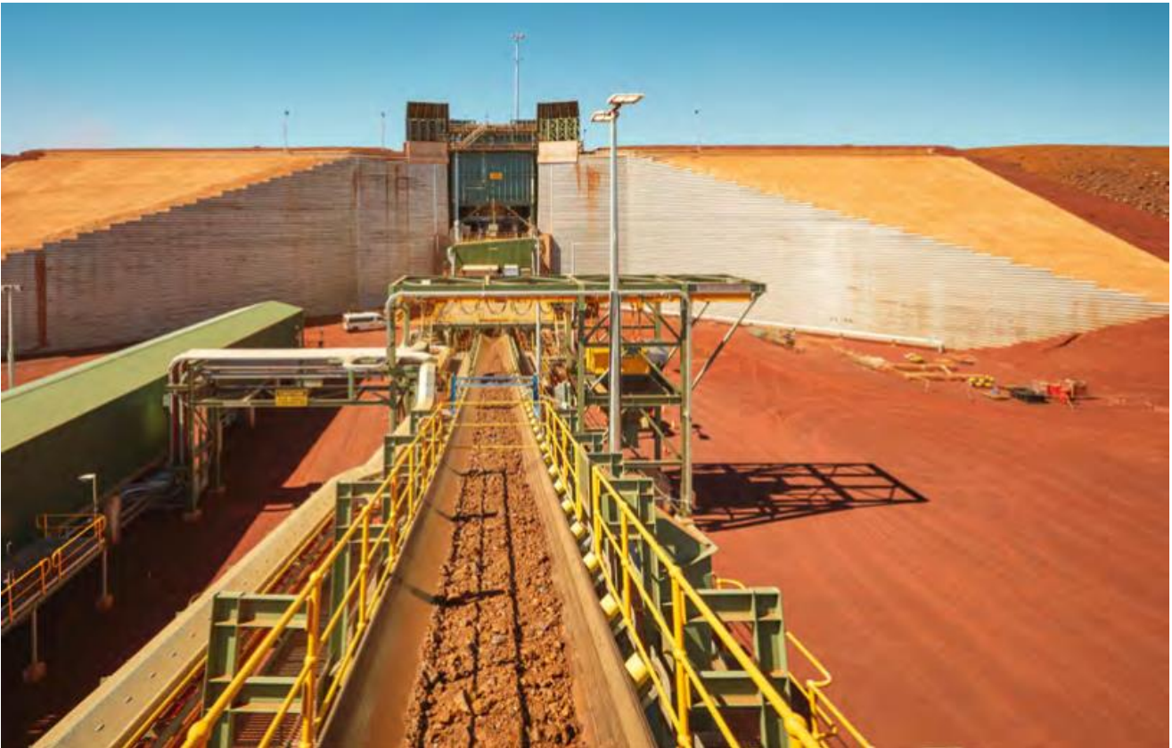
Ore leaving South Flank's Primary Crusher 2, one of two at South Flank that are the largest in BHP.
